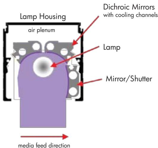
Mercury vapor lamps offer high efficiency at UV-A and UV-B wavelengths. But, as summarized in the figure at left, only about 10-20% of the input electrical power is delivered to the print medium as UV-A and UV-B radiation. The rest is lost as IR (infrared) radiation and heat. Heat is removed by forced-air cooling of the lamp and by air or water cooling of mirrors and other components in the Lamp Housing.
